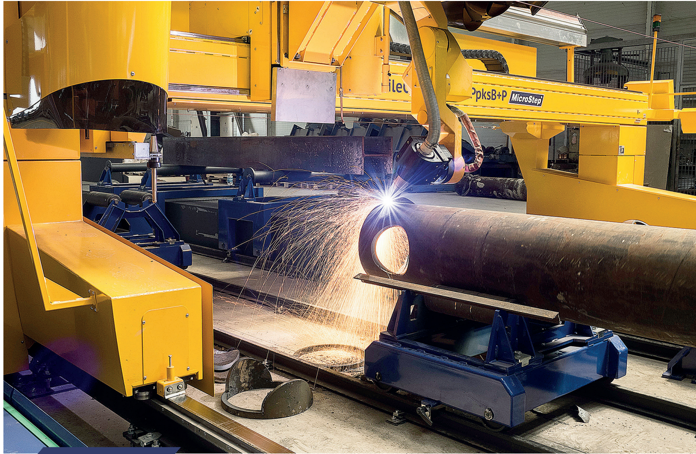
↑ MicroStep provides 3-D beveling with its patented auto calibration of tool geometry technology as well as a rotator beveling head.
