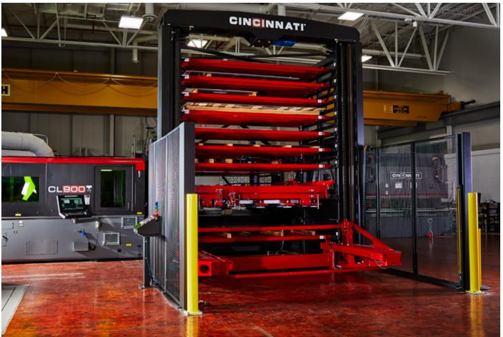
According to the team at RC Industries, the CL-900 fiber laser from Cincinnati Inc. coupled with a March automation system is as productive as two and a half  $CO_2$  laser machines.
