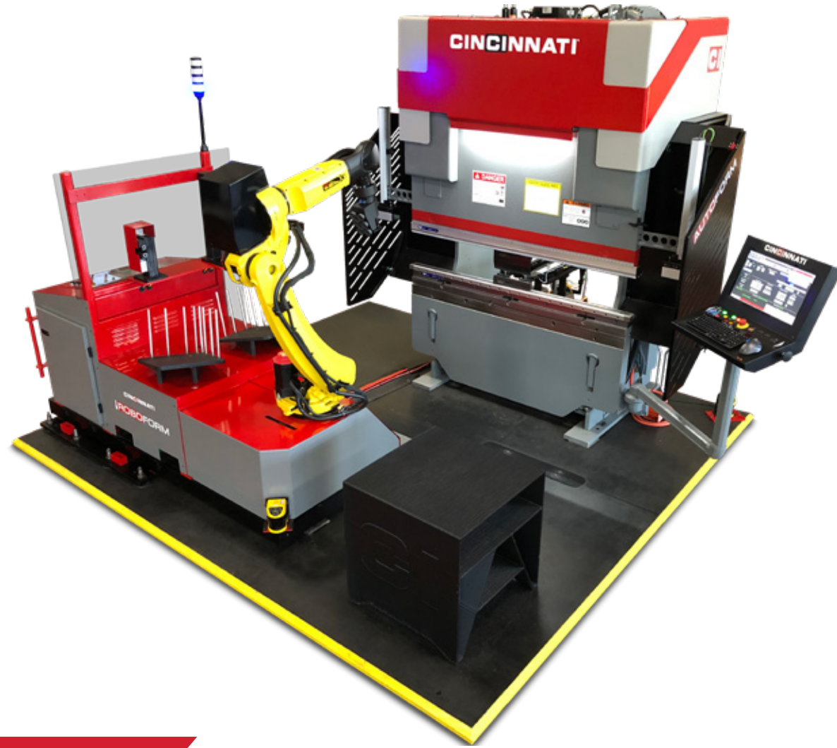
↑ Cincinnati Inc.'s RoboForm is an automated bending cell that was developed to allow bending operations to continue when human operator resources are limited.
