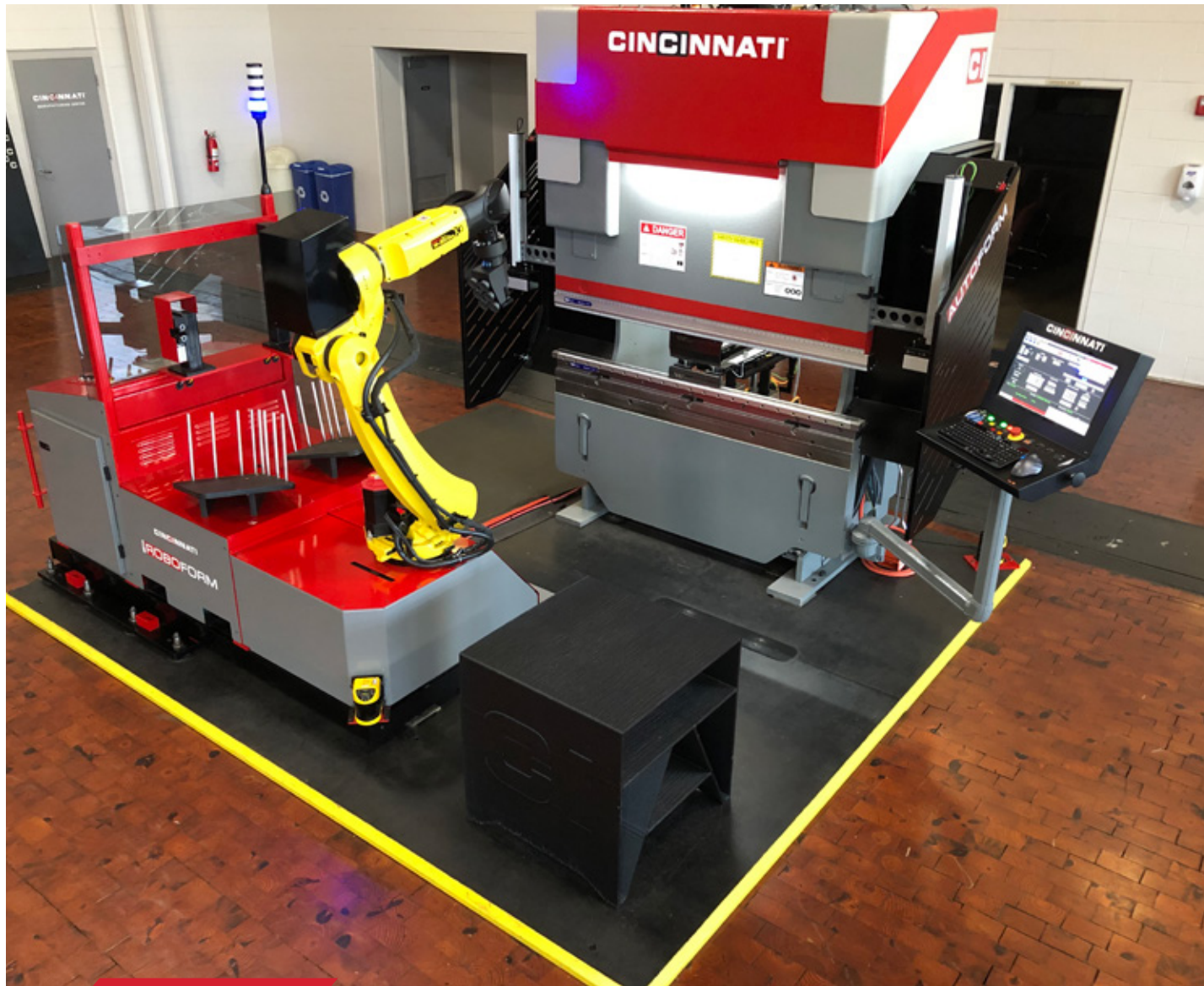
↑ The RoboForm automated bending cell with outbound tables paired with a 60-ton Autoform press brake on a safety platform.
