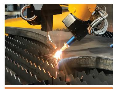
Oxyfuel rotator for weld preparation on thick metals utilizes MicroStep's patented ACTG technology for automatic compensation of kinematic inaccuracies, and thus delivers reliable cutting results in the long run with less frequent maintenance necessary.
