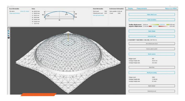
mCAM, the 3-D CAM software from MicroStep, maps the ideal cutting path onto a scanned object.
