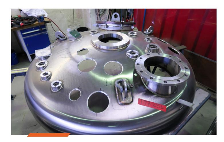
Dome cutting is used to create openings in the dish end of vessels, such as the one shown here, to facilitate the welding of inlet pipes and to prepare the end to be welded to the vessel body.
