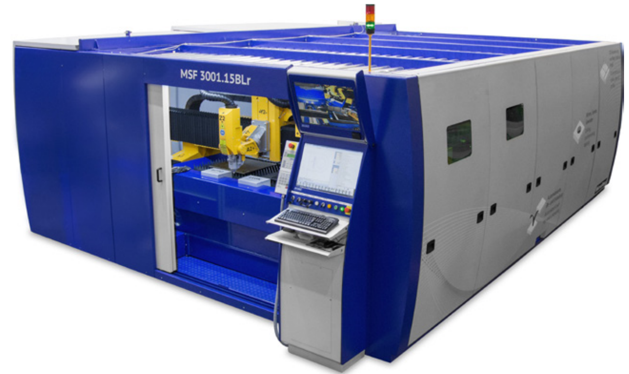
↑ The versatile MSF Pro is a powerful laser cutting system for processing flat sheet in 2-D (straight) and/or 3-D (bevel) as well as pipe cutting.
