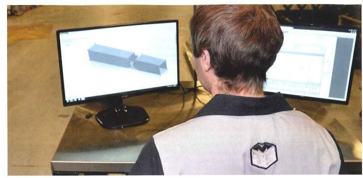
The Metal Shop's principal laser operator, Michael Cousins, uses SigmaTUBE software from SigmaTEK to develop a V notch. The right-hand monitor shows the positioning and cutting instructions for the laser machine; the left-hand monitor provides a graphical representation of the cut tube.
