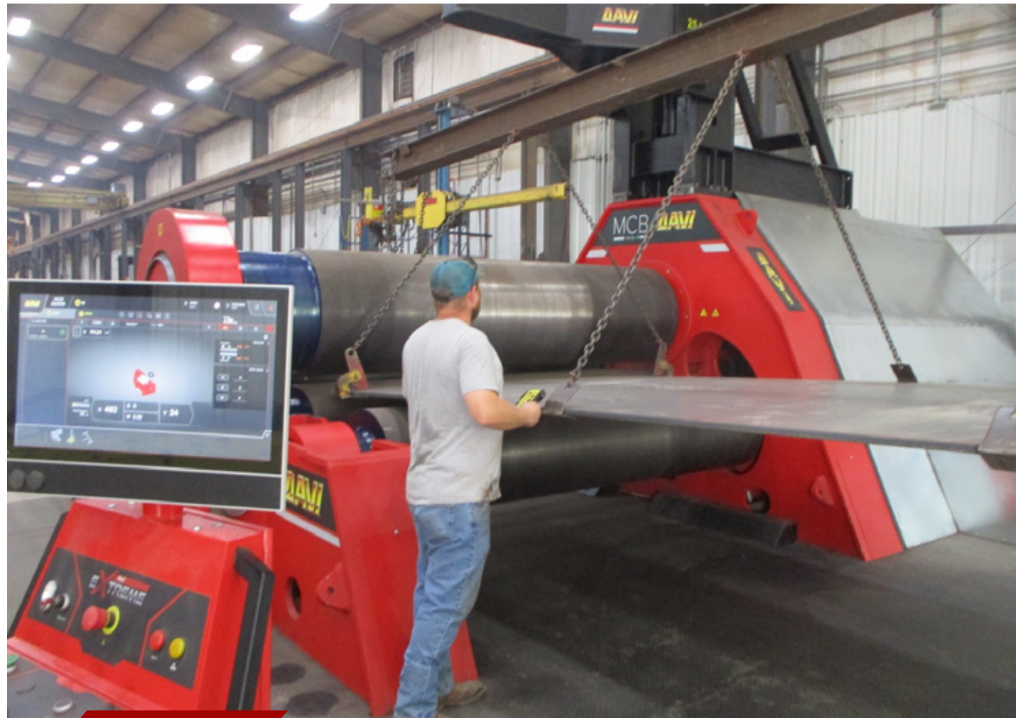
↑ Waterford Tank & Fabrication’s Davi MCB-T30 plate roller features a bottom roll that clamps thick plate, which guarantees operators precise control throughout the forming processes.
