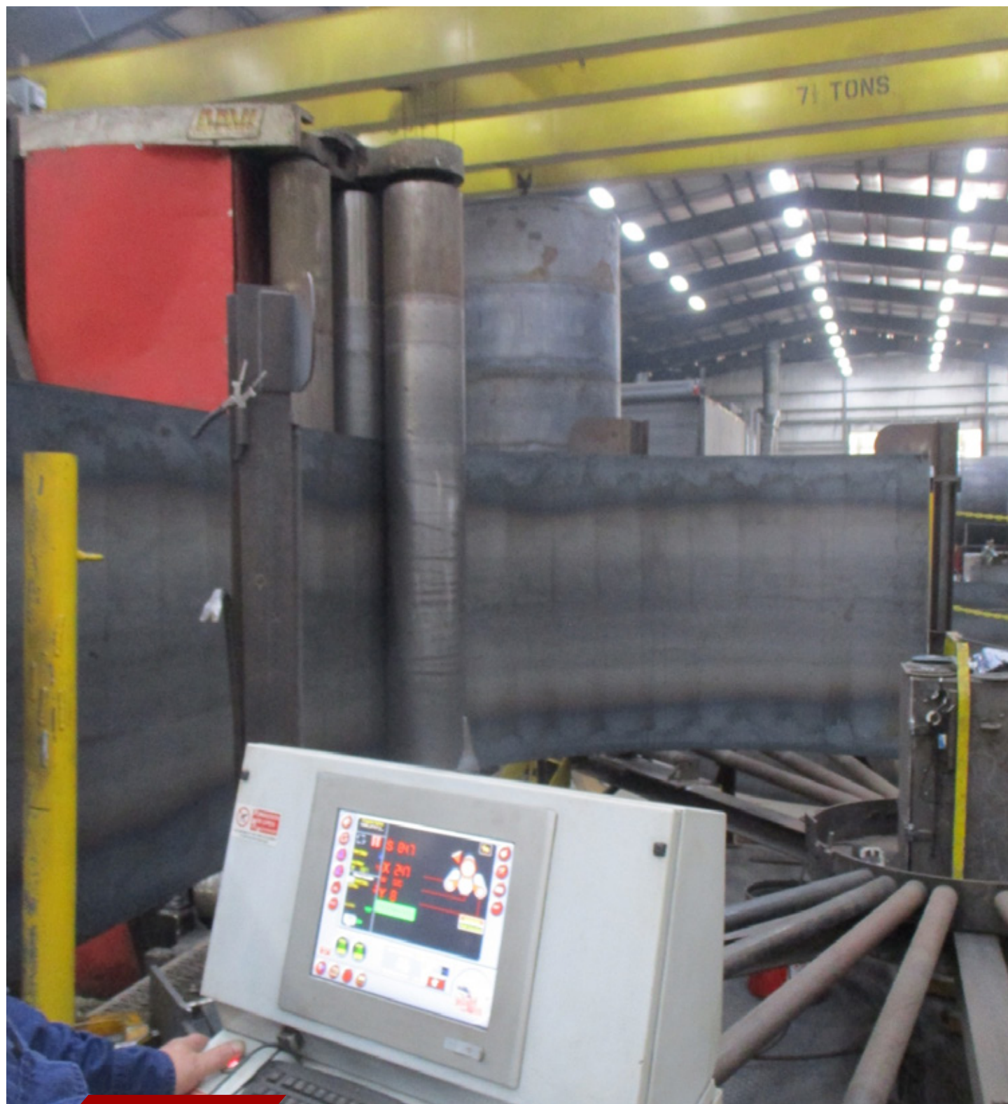
↑ Davi's iRoll eXtreme control system features a high-resolution touchscreen that includes intuitive 3-D graphics similar to a smartphone.
